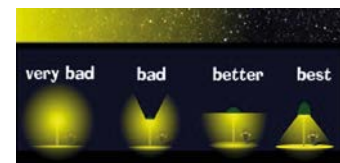
Note how the person standing under the light becomes more visible the more light is directed downwards
